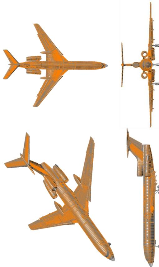
**Figure 1.4 Tu-154M FEA model and Building Block approach for full aircraft FEA model verification**
