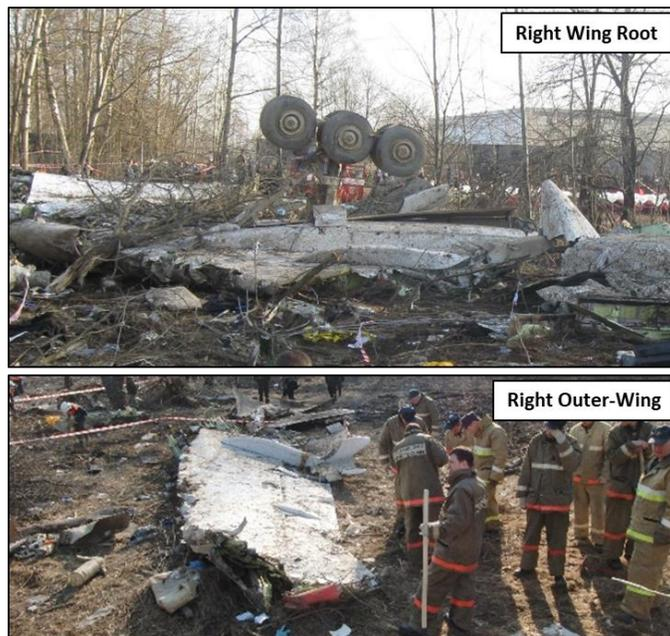
**Figure 4.25 PSC large debris images – Right wing [ 6 ]**
